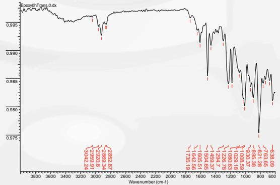
Figure 1. Non-exposed FBE FTIR spectrum
